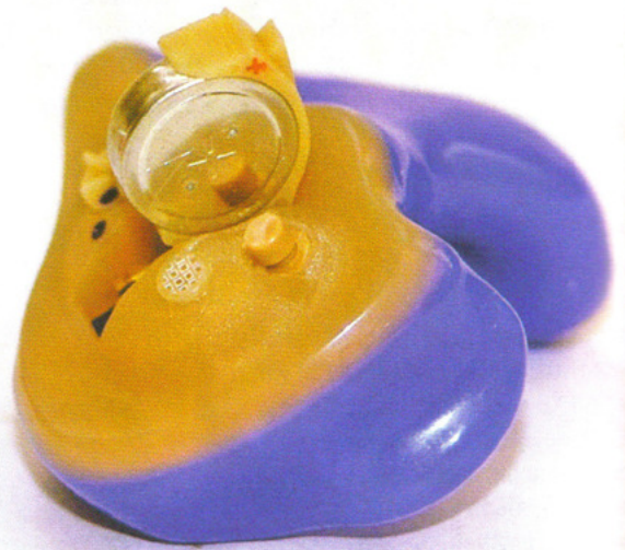
Detail of the plug; note the controls, microphone cover and battery compartment in its open position
